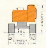
Operating weight (with standard 610mm (24 in.) shoes) Short arm and 0.7m3 bucket 18.2 t (40,040 lb.) Long arm and 0.7m3 bucket 18.3 t (40,260 lb.)
